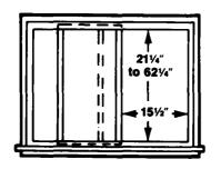
1. Unpack mounting parts before installing your air conditioner. Make sure you have all the necessary parts. A normal installation can be made with a screwdriver, saw, small level, pocket knife, tape measure, drill and 1/6," %64" and 3/16" drill bits.
